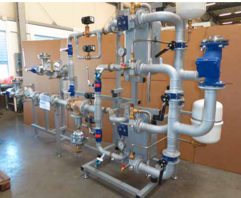
The ewers plant 1 for feeding in the heat from the Bochum district heating network
