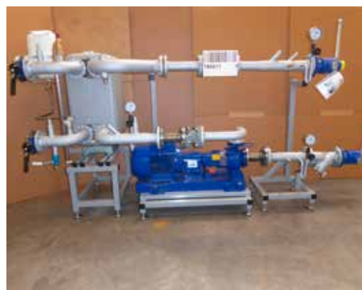
The ewers plant 2 for feeding back directly at the CHP unit
